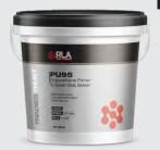
RLA PU 95 is moisture curing polyurethane primer and green slab sealer/ vapour barrier for cement-based substrates that are not subject to rising damp, or hydrostatic pressure. It can withstand a relative humidity moisture content up to 95% RH (ASTM F2170) it is a one component polyurethane primer/ green slab sealer that hardens and cures with the humidity present in the air and the substrate.
