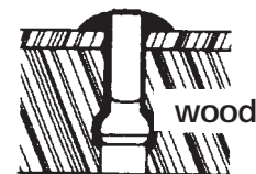
GROOVED RIVET Grooves improve holding strength
