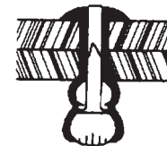
MULTI-GRIP PLUG One rivet does a number of grip ranges
